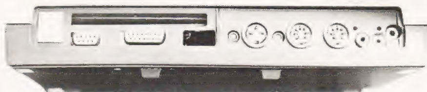
Rear view of an MB NewBrain exposing all the various I/O connectors, the bus port and the missing socket.
